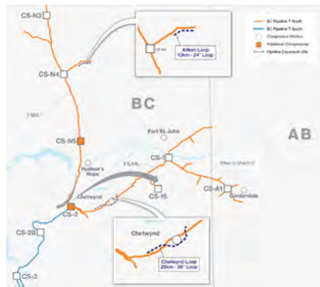
Figure 22: Spruce Ridge Extension pipeline loop extensions.
