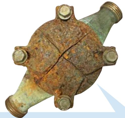
An improperly insulated water meter can result in a cracked meter in residences where the water meter is located in an unheated area.
