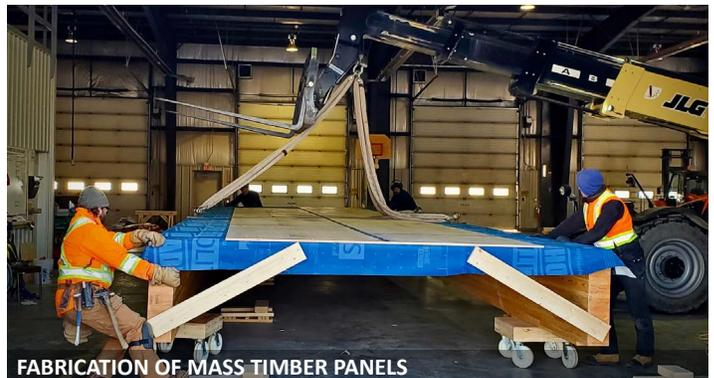
FABRICATION OF MASS TIMBER PANELS
