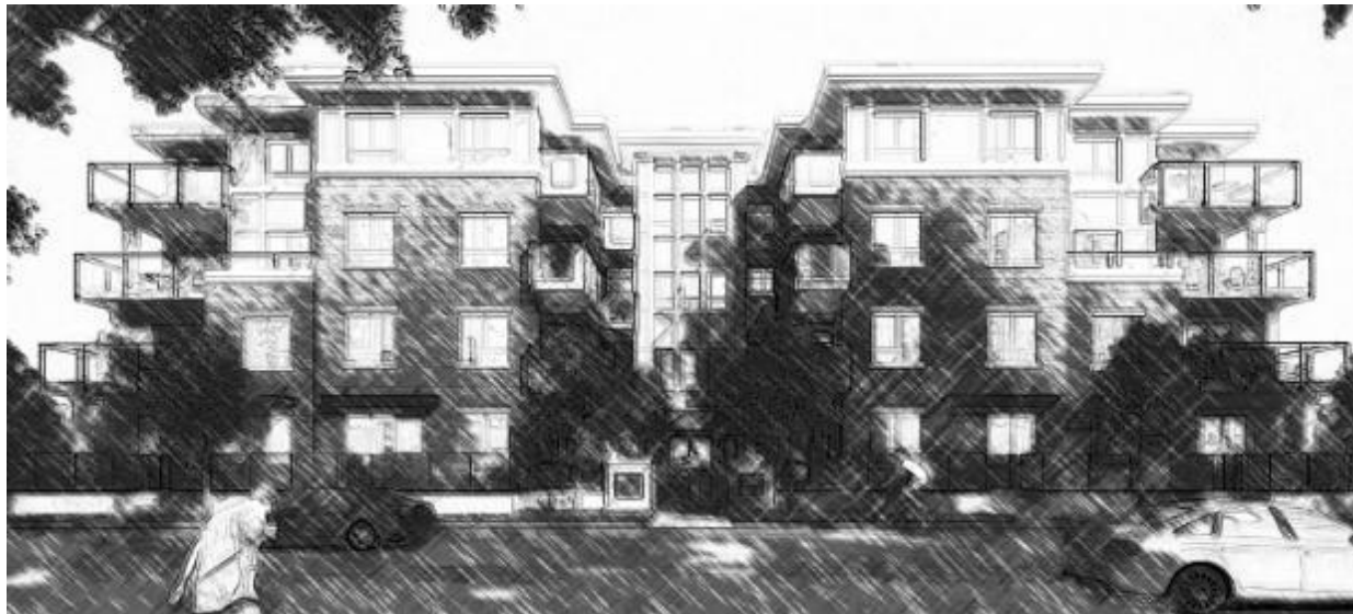
Figure 29: Demonstration of multiple storey building stepping back
